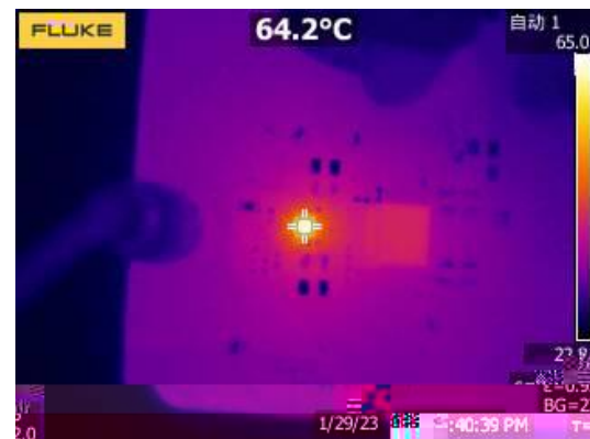
Figure 23. Thermal, 12VIN, 5VOUT, 3A
